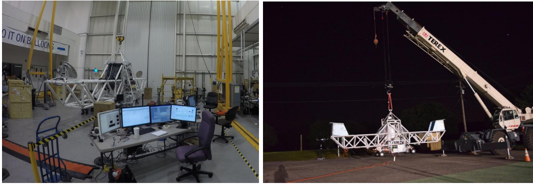
Figure 2.4: Indoors and outdoors hanging tests of BETTII
