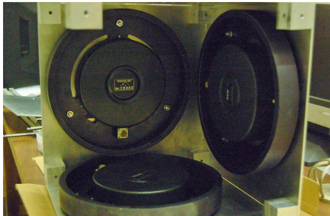
Figure 1.6: The three SRS-2000 gyroscopes mounted in an orthogonal assembly.
