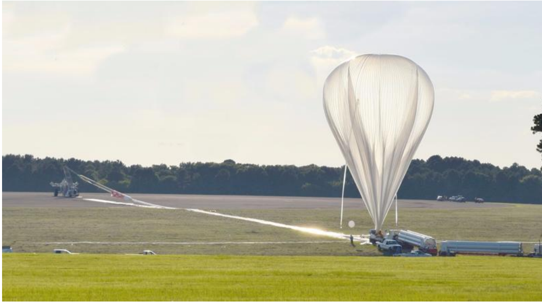
Figure 2.1: BETTII balloon launch. On the left, the payload is captured by the launch vehicle "Big Bill", until the balloon is inflated and released. The parachute assembly can be seen in orange, connecting the bottom of the balloon with BETTII.
