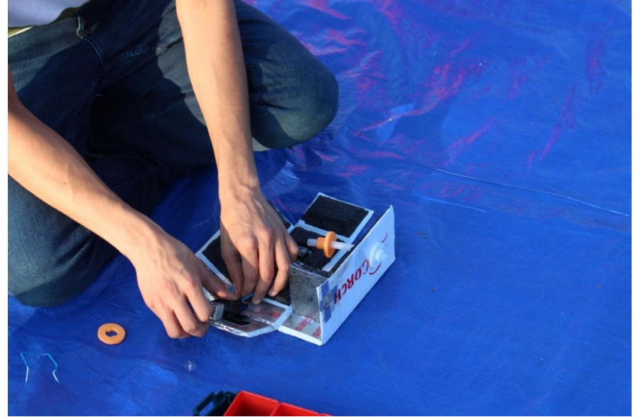
SCORCH - Uses a model rocket engine to burn a hole in the payload string
