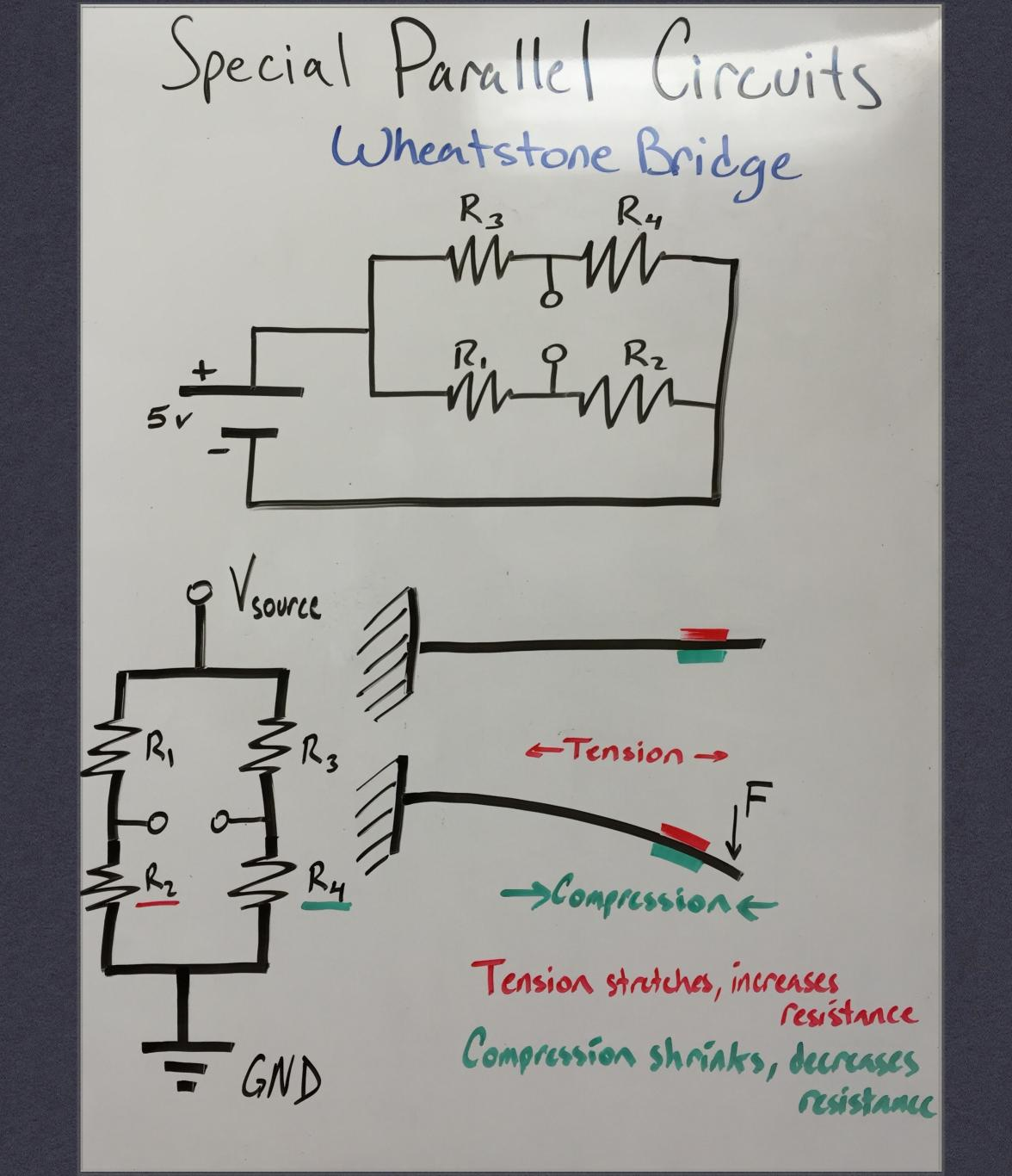
Special Parallel Circuits Wheatstone Bridge 9 Vsource  $V_{source}\left(\frac{R_2}{R_1 + R_2}\right)$ ŽR3 ZR,  $5\left(\frac{98}{100+98}\right) = 2.475v = V_{1}$ Ry Vsource  $\left(\frac{R_3}{R_3 + R_4}\right)$  $5\left(\frac{102}{100+102}\right) = 2.525v = V_2$ GND  $V_2 - V_1 = 0.05$  volts
