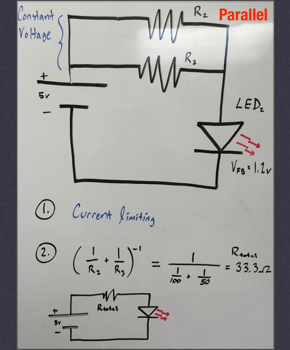
Equivalent Circuit Para le Rtotal = 33.3.2 5.0 5√ Constant Current  $V_{FB} = 1.2v$ 3.  $(V - V_{FB}) = (i)(R_{total})$ (5-1.2)=(i)(33.3.2) $i = \frac{3.8r}{33.3\Omega} = 0.114 \text{ Amps}$ i = 114mA
